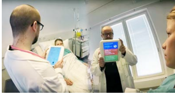
Fig. 1. The dual-sided tablet used in a hospital context. The front display shows electronic health record information, whilst the rear display provides the patient with visual information to support the consultation process.
