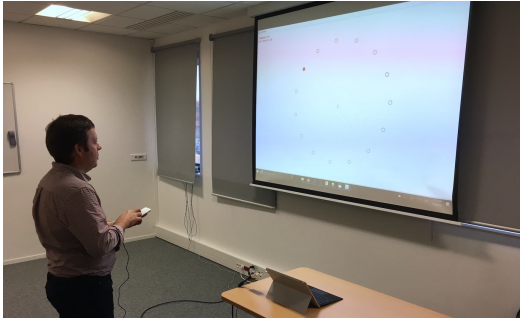
Figure 3. Illustration of the experimental setup: participants stood 2 meters away from a rear-projector screen. The input device was connected via USB to the computer in order to guarantee stable data transfer for smooth control.
