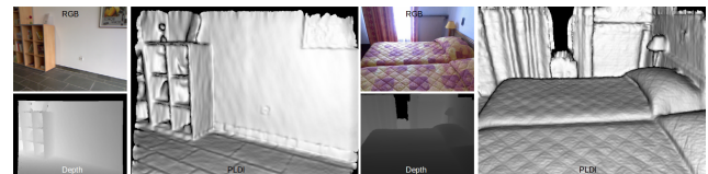
Figure 2. Example RGB-D scenes and corresponding PLDI images. Photometric features emerge along the floor (tiles), library (wood texture), poster et blanket covers. Depth gradients are noticeable along the wall and the double beds.
