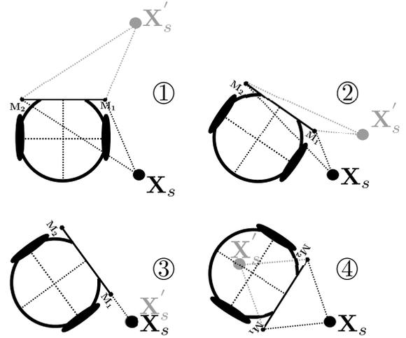
Fig. 5: Facing a sound source located behind: the robot moves with respect to the phantom sound source  $\mathbf{X}'_s$  (steps ① to ③) instead of  $\mathbf{X}_s$  until reaching a configuration where  $y_s > 0$ .
