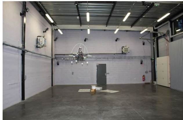
(b) The Pelican UAV in the VICON area. The flying area available is 15 \times 10 \times 5 \text{ m}^3 equipped with twenty T40S Vicon cameras.
