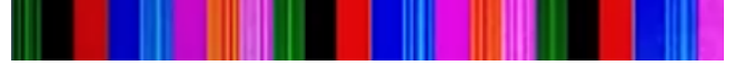
Figure 5. The 8-CSK modulation symbols combined with a 20 kHz PWM on the green channel only.
