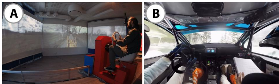
Figure 2. Simulators using ODV content. A: A road grader simulator where the video is projected on the wall using three projectors. B: Rally car simulator used with a VR headset.
