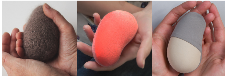
Fig. 1. Evolution of coating: knitted from wool (left), sewed from an elastic material (middle), easily exchangeable pattern sewed from an elastic material (right).
