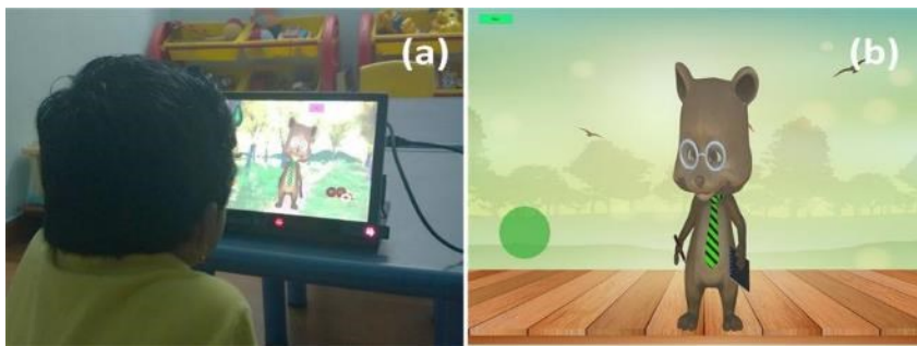
Fig. 3. (a) Experimental setup. (b) A frame from the interactive introduction of the Little Bear gaze-aware agent. The green dot indicates the current gaze point of the user.
