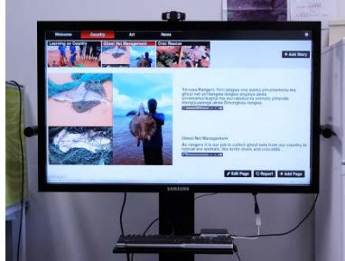
Fig. 2. A working prototype of the Digital noticeboard shown on a wide touch screen mounted on wheels. On the shelf below the screen is the Intel NUC mini PC that runs the noticeboard: this is the 'package' that is shipped for deployment.
