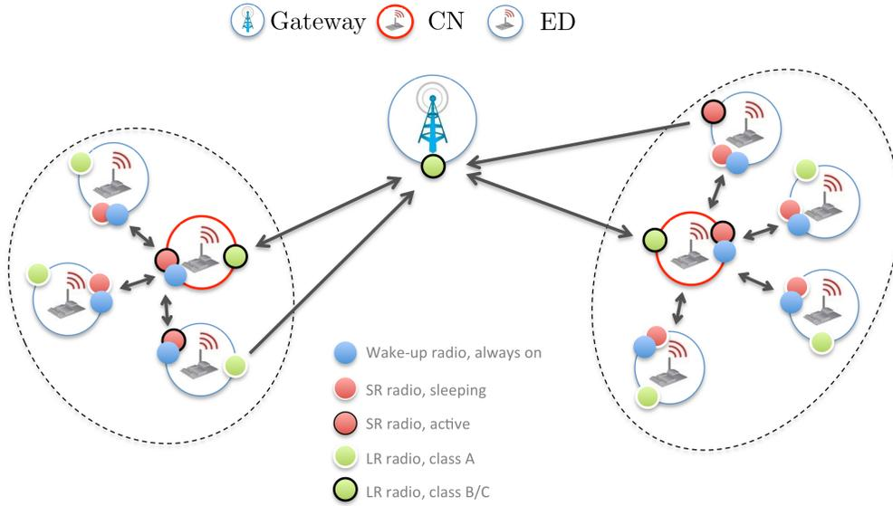
Fig. 2: Cluster-based network architecture for Long-Short range communication.
