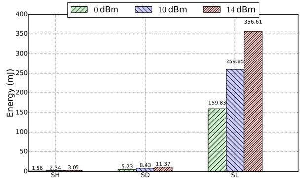
(a) Energy cost of sending a packet using LoRa™.
