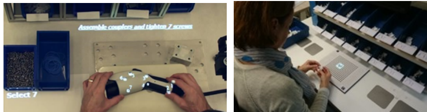
Fig. 1. Flexible operator support system with instruction projection.
