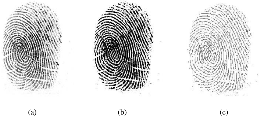
Fig. 2. Original image (a) image after binarization procedure (b) and image after thinning procedure (c).
