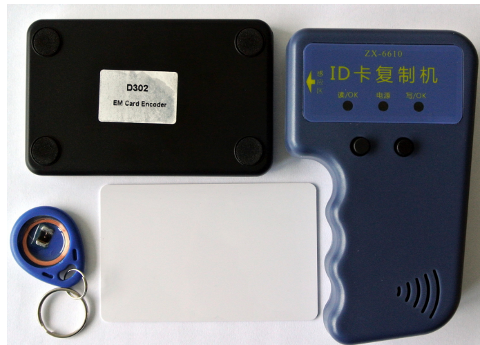
Fig. 3. Cloning of EM proximity 125 kHz tokens – from top-left corner clockwise: a USB writer, a hand-held copier, a blank card and a blank tag (with protective cover removed)
