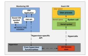
Fig. 2: A Typical VMI Architecture [30]
