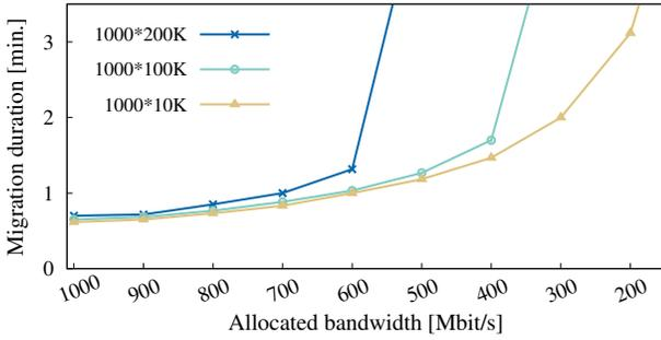
Fig. 3. Duration of a live-migration between 2 KVM hypervisors depending on the allocated bandwidth and the parameters used by the command *stress* to generate dirty pages. *1000\*10K* indicates the VM runs 1000 concurrent threads that continuously allocate and release 10 KiB of memory each. The VM memory used is set to 4 GiB and the downtime is limited to 30 ms.
