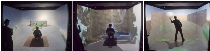
Fig. 4. The tasks in the DAVE; from left to right: Task 1 - Observation: The participants were asked to find a specific part of the machinery by observing the scene; task 2 - Emotion: The participants had to ride a roller coaster; task 3 - Interaction: In a mini game the participants had to catch balls shot in a random angle at them.
