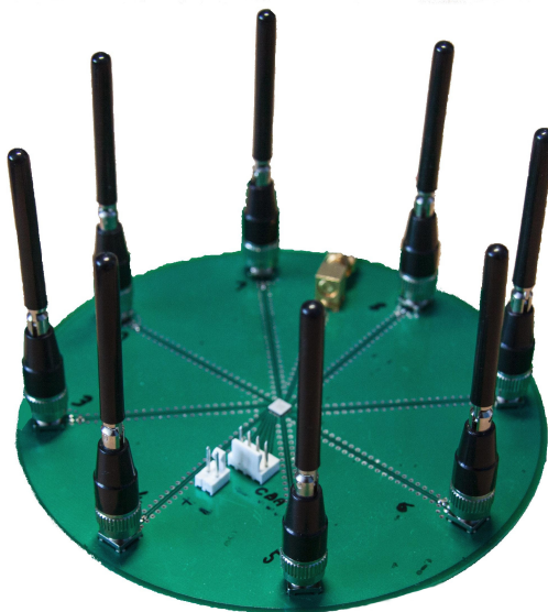
Fig. 2. Pseudo-Doppler antenna array
