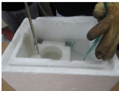
Fig. 4. Totally submerged stator in LN 2 .
