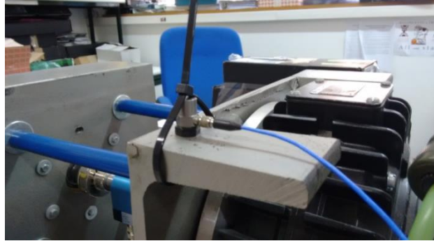
Fig. 4. Transversal vibrations measuring using an accelerometer.
