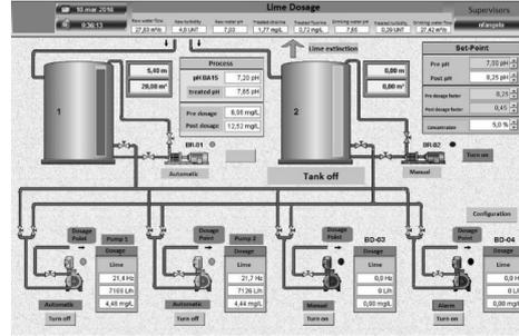
**Fig. 1.** A process screen in the SCADA system for pH monitoring and lime dosage
