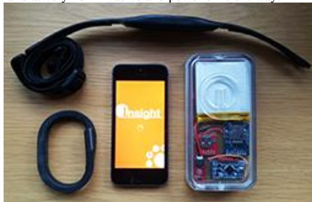
Fig. 3. Data collection using Jawbone UP, chest-strap heart monitor, data-logger and app
