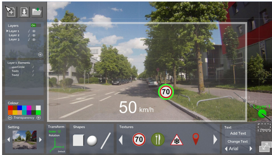
Fig. 2: The 3D-HUDD allows to create the visual layout of an head up display in front of a static 3D scenario.
