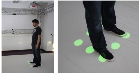
Fig. 10. Alternative floor display using a ceiling-mounted short-throw projector.
