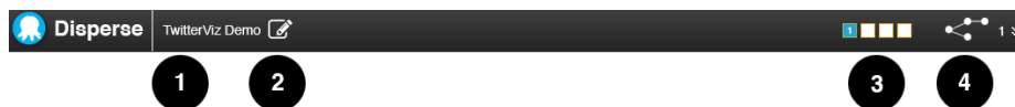
Fig. 4. The Disperse interface appears as a header in each browser window and includes (1) the name of the visualization that is being run, (2) a source code editor, (3) the screen layout, and (4) a branch selector.
