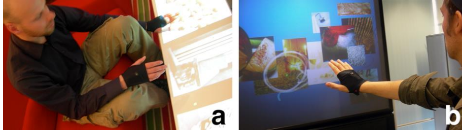
Fig. 9. a) In the Funky Coffee Table, designers use their hands to store images in layers above the table. b) Funky Wall uses hand gestures, body position, and speech to support presentations.
