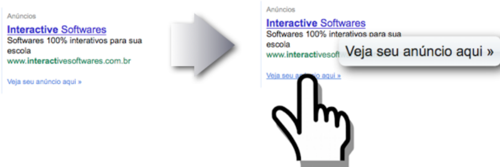
Fig. 1. Outline of the link-offset-scale functionality: as the user positions his finger over a specific link (touching the display), the browser presents the content of that link in a separated magnified element next to the user's finger, so as to be in his field of view.
