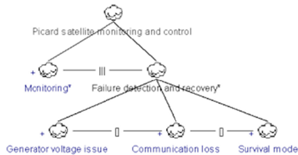
a) Top-view of controllers’ tasks, including Monitoring and Failure detection and recovery
