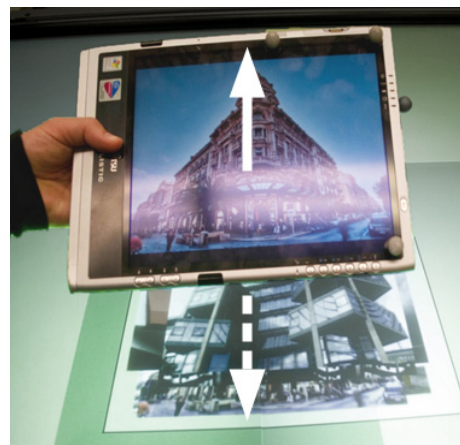
Figure 5. Browsing stack of photos by holding and moving a tablet computer.
