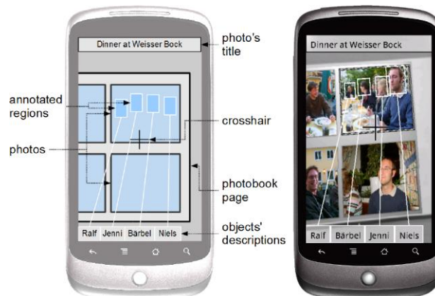
Fig.2. The design shows the annotations aligned to the display's top and bottom. Only the annotations of the photo below the crosshair are visible.
