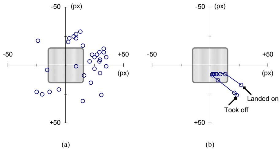
**Fig. 7.** (a) Due to repetitive overshooting, a participant touched the screen 32 times to tap a small target (P12, Week 2). (b) Adding extra pressure (i.e., "pressing") on the screen while tapping can cause an irregular trajectory (P13, Week 2).
