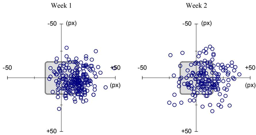
**Fig. 6.** The distribution of touch locations relative to the location of the 30-pixel target on the small device before and after a week's practice. The target area is shown as a rounded square. The participants tended to tap the right side of the target. The variation of touch locations was larger after the week's practice.
