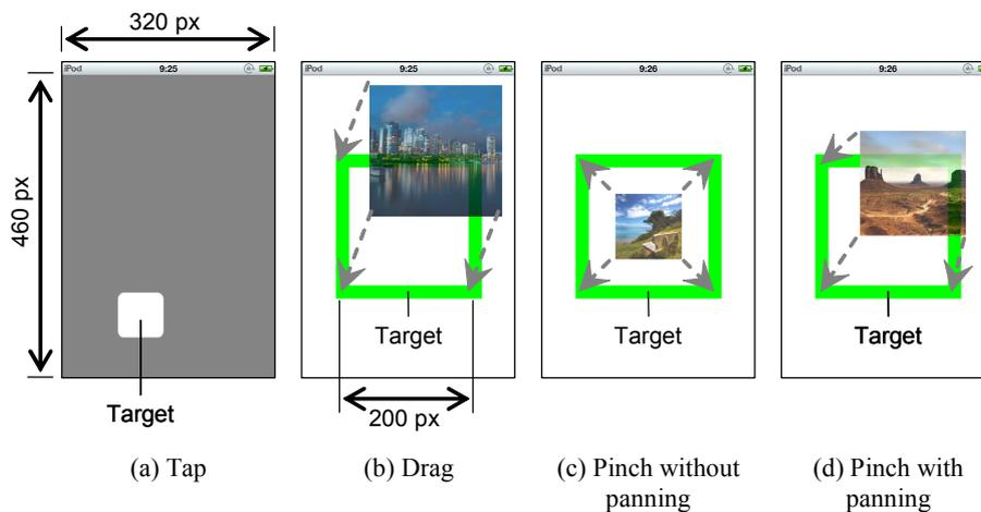
**Fig. 1.** Our experimental software was designed to practice and assess four standard touchscreen operations: (a) tapping, (b) dragging, (c) pinching without panning, and (d) pinching with panning. The text, lines, and arrows are annotations, not displayed in the actual experiments.
