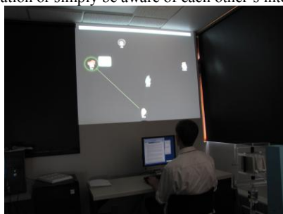
Figure 3. A user seated in front of an OMNI display, with four remote contacts. The user is focused on the leftmost contact, as indicated by the line.
