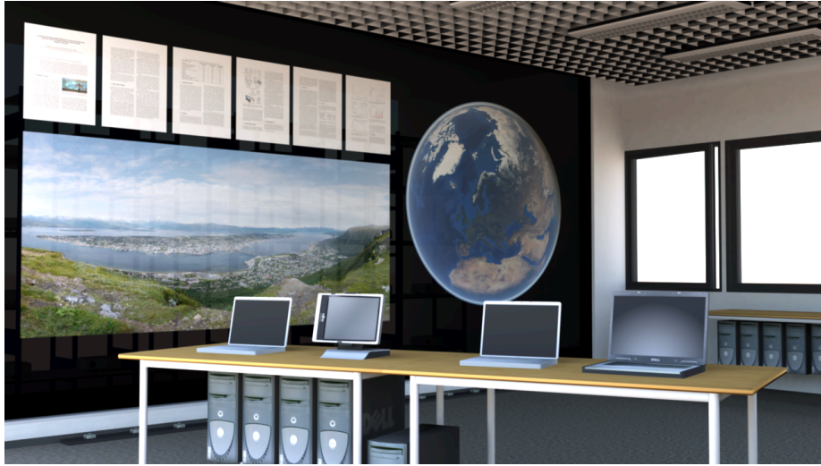
Fig. 1. Illustration of multiple desktop computers used as a NAC resource to provide processed data for a visualization system running on a high-resolution tiled display wall.
