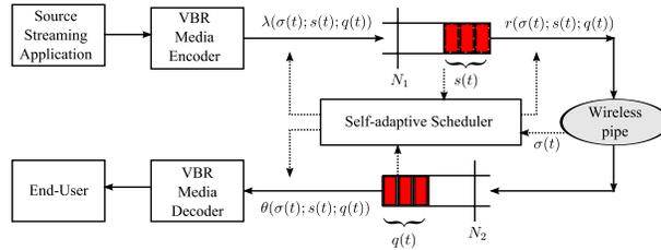
**Fig. 1.** The considered battery-powered wireless streaming system.
