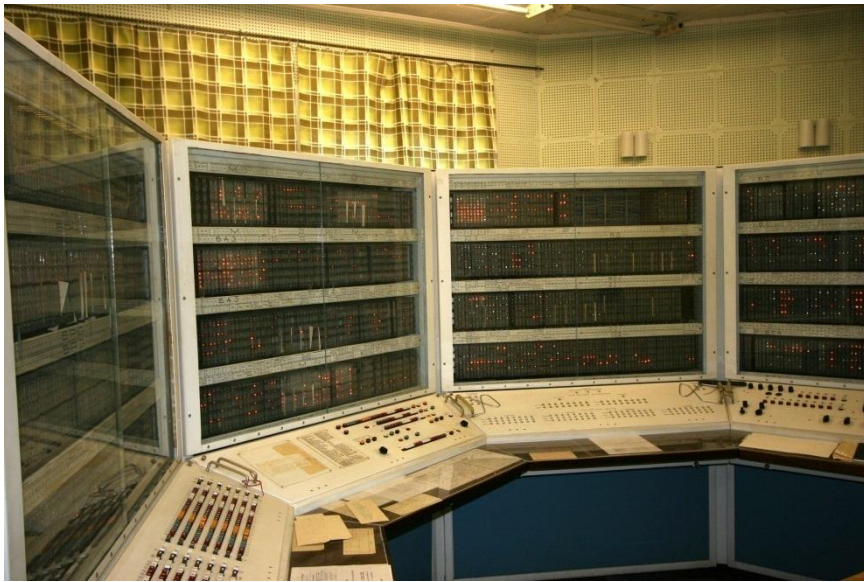
Fig. 1. Front view of the BESM-6 central processing unit.
