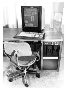
keyboard is set on a pull-out frame located underneath the desk surface and allowing configuring position and angles. The keyboard had 137 buttons, 134 of them fully pre-programmable; that is, a driver defines their layout and semantics.
