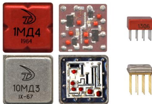
Figure 7. First series IC in the USSR, “Tropa”, thick-film, a top number, “Posol”, thin-film, the bottom number. (At the left and in the center – in the double size, on the right – in full size).
