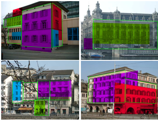
Figure 11: Example of failures with different cases of false detections (images 1, 2 and 3) and matching failure with two different facades matched to the same reference (image 4)
