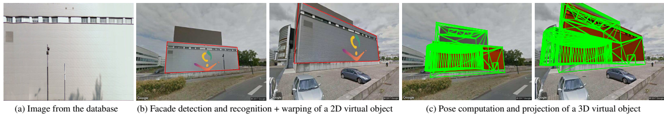
Figure 1: Facade proposals for Urban AR. A facade of the Nantes Event Center building (a) is automatically detected and recognized in two views of the building (b, red polygons). From these results, any planar virtual object added to the facade (here the ISMAR logo) can be warped according to the transformation of the facade. (c) When some geometric information about the facade is available, any 3D virtual object expressed in the same reference frame as the facade (here the ISMAR building) can be added to the view.
