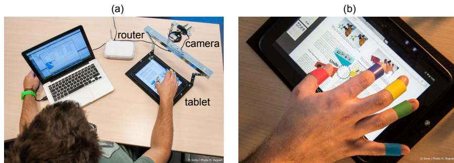
Figure 13: Finger identification technique used for the tablet and smartphone: (a) a camera is mounted on a frame fixed to the tablet or smartphone; (b) coloured rings are attached near each finger tip.
