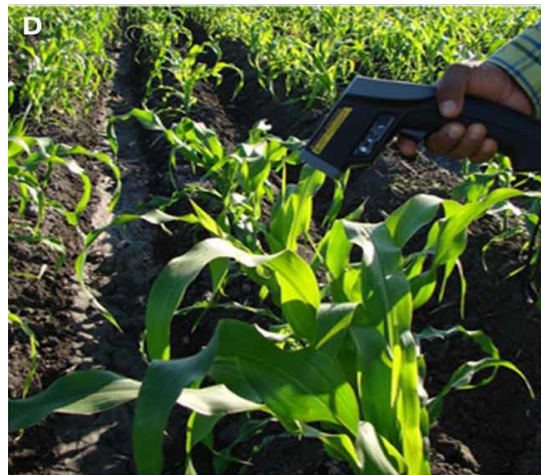
Fig. 2. Canopy temperature measured by infrared thermal imager
