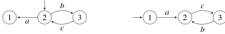
Fig. 6. SPA G (left), and DFA G^R for the reversal of the language L(G) (right); projection P : \{a, b, c\}^* \rightarrow \{a, c\}^* .
