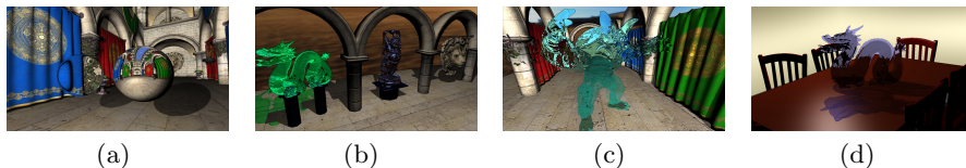
Fig. 5. Images rendered with our hybrid ray tracer implementation. (a) Sponza Atrium Scene. This scene highlights the real-time reflection and refractions effects. (b) Showcase Scene. In this scene we highlight the colored shadows of transparent objects. (c) Armadillo Scene. This is demonstration of a refractive material applied to a model. (d) Dining Room Scene. All images have a resolution of 1280x720 pixels.
