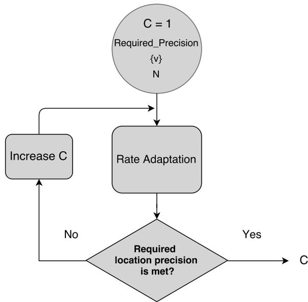
Figure 11: Block diagram for dynamically provisioning LTE resources.
