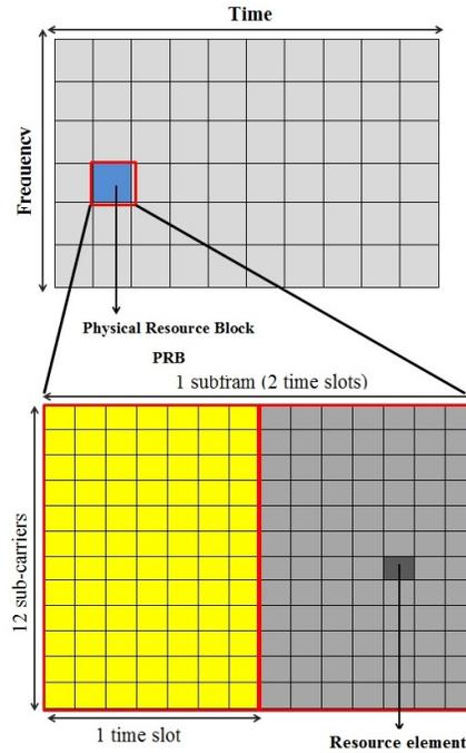
Figure 2: Physical Resource Block (PRB) within LTE.
