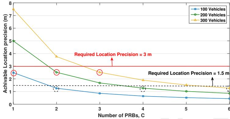
Figure 12: Sizing the number of required PRBs.
