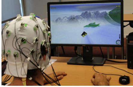
Figure 1: Participant using MI commands to play TuxRacer, e.g. imagining right hand movement to catch fish on the right.
