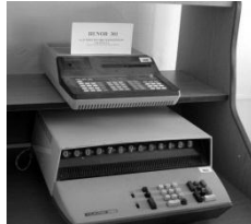
Figure 9.2: Hunor 131. Electronic table calculator
