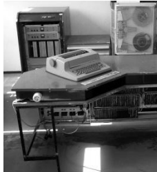
Figure 9.3: The control desk of the EMG 830 computer
