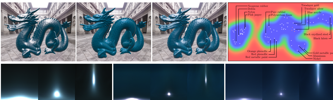
Figure 3: Real-time exploration of our BRDF manifold. 3 materials (red points) are chosen manually, in the vicinity of blue-acrylic , by clicking in the 2D latent space (top right). The latent variables were optimised using all 101 materials of the MERL database. Our proposed construction of the BRDF manifold lends itself to real-time rendering (25 fps) using interpolated materials along with all combinations of dynamic geometry, view points and lighting (see sec. 3.3) using zonal harmonics up to L = 40 [Soler et al. 2015]. The slices of the interpolated BRDFs are also visualised. Please see the accompanying video for a live demonstration.
