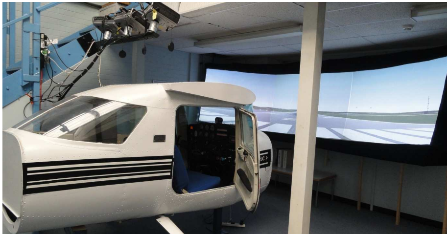
Fig. 2. Cessna 152 Cockpit Simulator (University of Hertfordshire)
