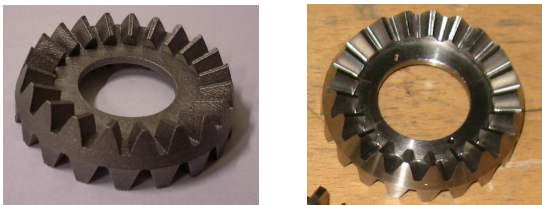
Figure 19: Example of mechanical component (a bevel gear) manufactured with AM (left) and with subtractive technique (right). The surface finish achieved by AM is not compatible with the specifications of the gear, so a finishing operation (e.g., by milling) is required.
