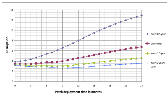
Fig. 5. Overall disruption when \alpha=10 and exploit development time is 1 year for different exploit arrival rates.
