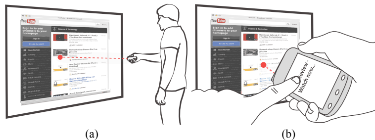
Fig. 8. Using the mobile phone as a remote control for browsing web pages on a TV set.
